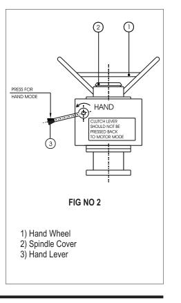
4) Bring the actuator output shaft in the 50 % position of the complete travel so that it can move freely in either direction. This can be done through Hand Wheel mechanism as detailed above.
