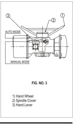
4) Bring the actuator output shaft in the 50 % position of the complete travel so that it can move freely in either direction. This can be done through Hand Wheel mechanism as detailed above.
